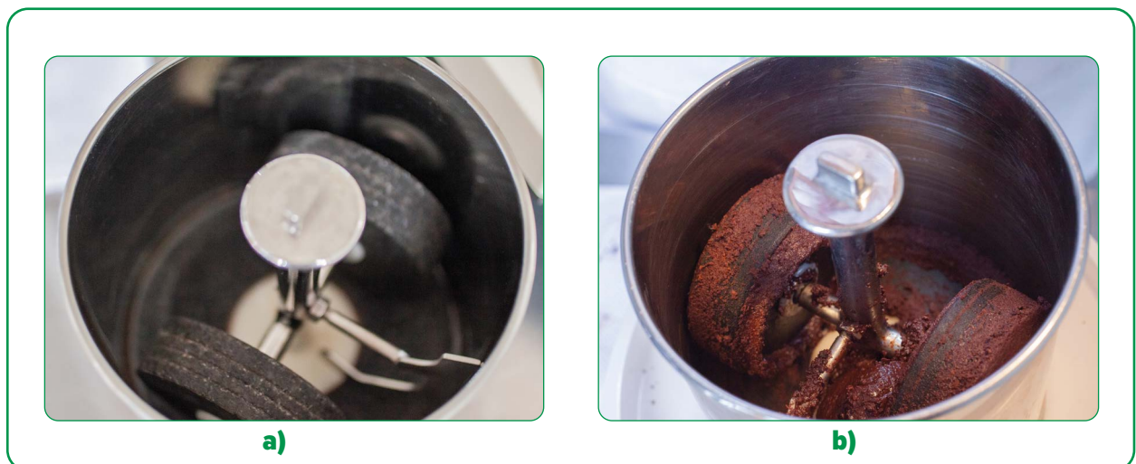
Figure 69. Inside the melanger: a) view of stone grinder assembly inside the empty stone bowl; b) view of the melanger bowl while grinding cacao nibs into cacao mass. ( chocolatemelangeur.com ; chocolatealchemy.com ).
