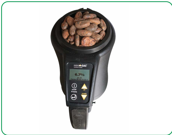
Figure 50. Dickey-John Mini GAC 2500 moisture metre with loader ( dickey-john.com ).
