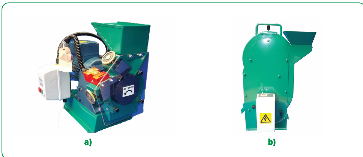
Figure 64. CAPCO stainless steel equipment for a) breaking and b) winnowing cacao beans ( capco.co.uk ).
