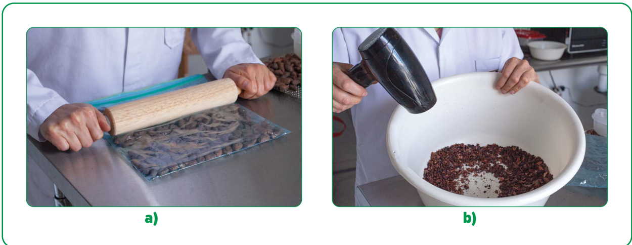
Figure 62. Semi-manual method of winnowing cacao beans. a) Rolling pin, b) hair dryer (Bioversity International, Archila, 2022).
